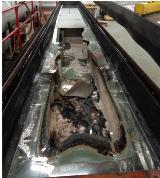
Photo No. 3 Unexposed Surface of the Test Specimen (Post-test)
